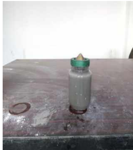
Figure 2: Specific gravity test of fly ash
