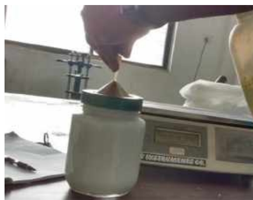
Figure 7: Specific gravity test of hydride lime
