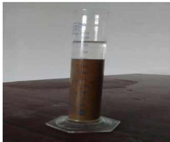
Figure 5: Silt test of the sand
