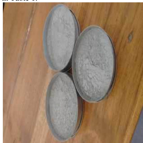
Figure 3: Moisture content test of fly ash
