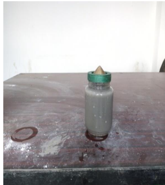
Figure 2: Specific gravity test of fly ash
