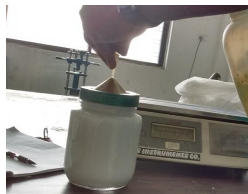
Figure 7: Specific gravity test of hydride lime
