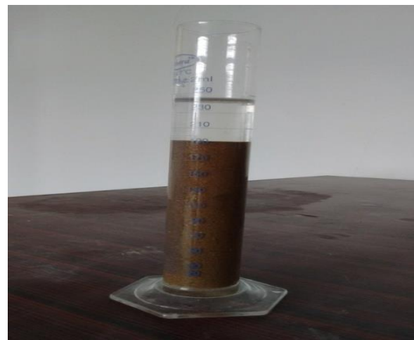
Figure 5: Silt test of the sand
