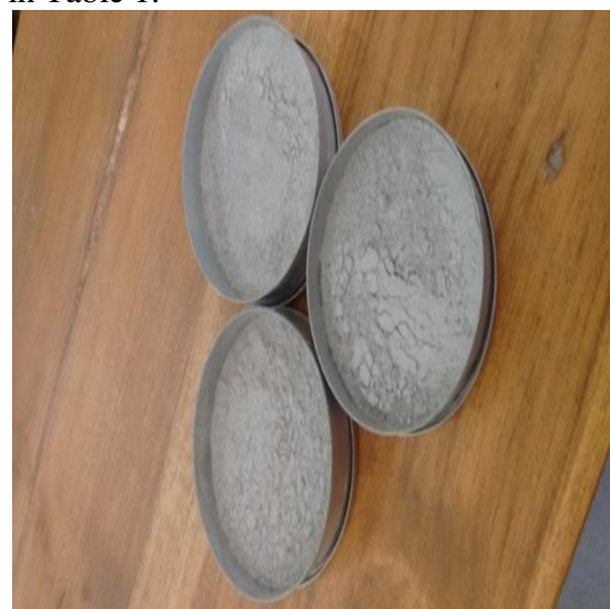
Figure 3: Moisture content test of fly ash
